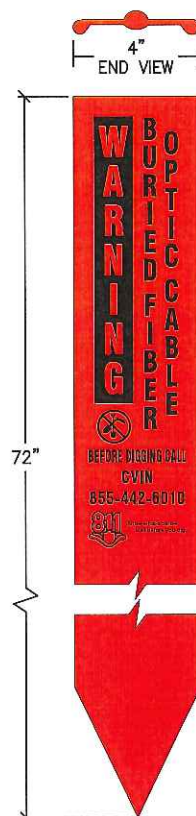
WARNING SIGN – RHINO 3 RAIL FIBER OPTIC CABLE MARKER NTS
